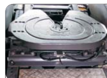
Practical example: fifth well support plate
