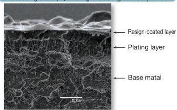
The treated surfaces are highly resistant to corrosion and can be widely used for places that require high corrosion resistance. The plated surface of a base metal is further coated with an acrylic resin layer. This reinforces the anti-rust property of the surface.
