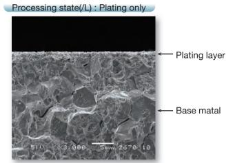
The deposited layers are hard to be separated and can have a long-lasting high anti-rust property. The plated layer is very thin (1 to 2  $\mu$ m), and superior to corrosion resistance to other plating methods. (Applicable to small L/W)
