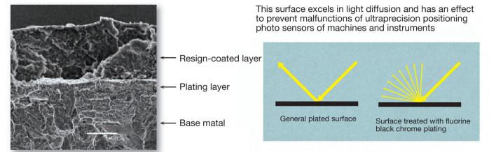
The black chrome surface is further coated with a difluoride resin. This makes the surface more highly functional. The surface-treated parts can be used as light-diffusing parts for ultraprecision positioning devices, etc. The deposited layers strongly adhere to the base material and have highly corrosion resistant, Solvent resistant and anticorrosion property. They are also very strong and consequently very versatile.
