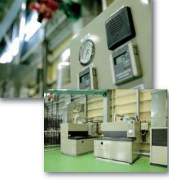
4 Coating system and baking furnace We have installed various kinds of apparatus to make coating layers as uniform as possible and a new gas baking furnace to shorten the baking time. (Improvement of coating accuracy and shortage of baking time)
