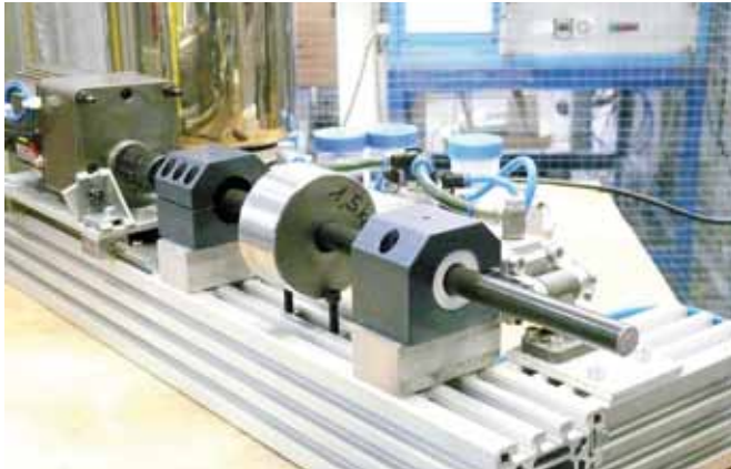
Picture 02: Test bench for xiros® polymer ball bearings at igus® laboratory
