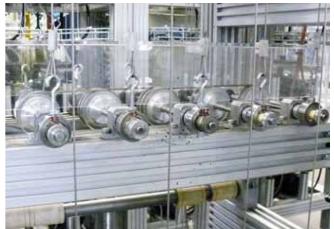
Picture 01: Test bench for xiros® polymer ball bearings at igus® laboratory
