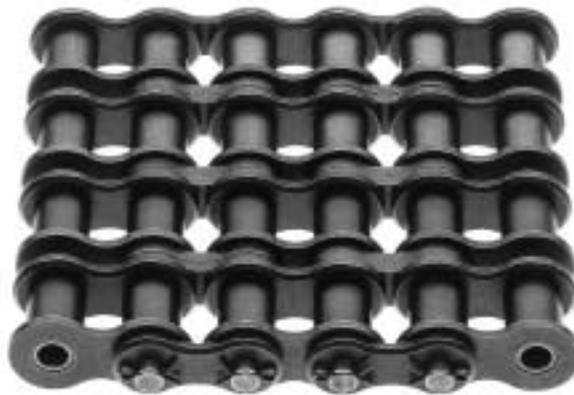
**Press-fit center plate:** Press-fit multiple strand chains were originally developed by Diamond for service in applications that require the utmost in multiple strand chain capacity. Multiple strand chains with press-fit center plates have significantly greater fatigue strength than their slip-fit center plate counterparts, because press-fit construction assures rigid, permanent support for the pins at each tension point with no relative movement, which can cause wear or fatigue.
