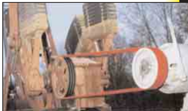
Oil Pumping Unit: 3 x "C" section—Handles shock loads, resists dry rotting and provides on-site availability.
