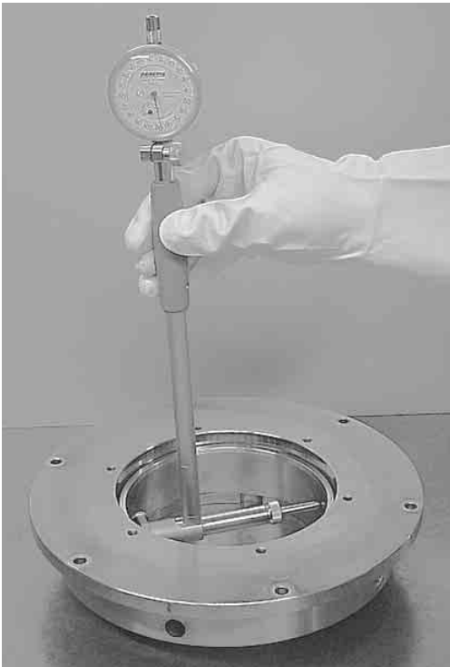
Fig. 1.10 Zero Setting of Cylinder Gauge
