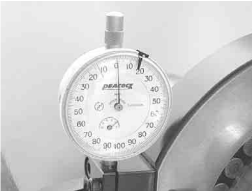
Fig. 1.15 Measurement of Spacer Width
