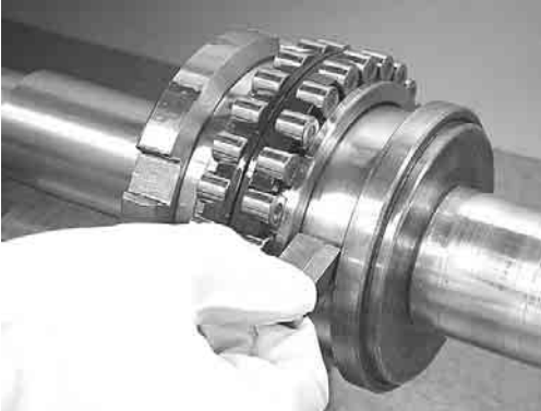
Fig. 1.15 Measurement of Spacer Width
