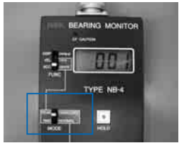
Recording of vibrations caused by a scratch inside a bearing (ENVELOPE)
