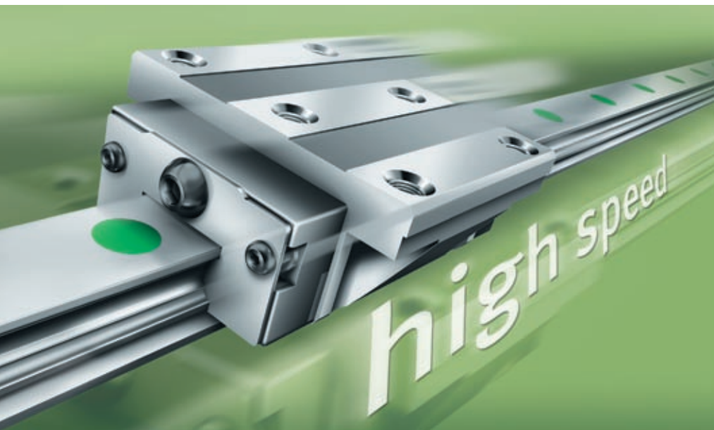
High load carrying capacity and rigidity and speeds of up to 10 m/s: Four row high speed linear recirculating ball bearing and guideway assembly
