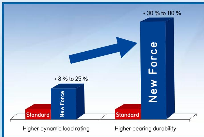
Higher dynamic load rating enables clients to lay out smaller dimensions designs to carry identical load. Thus ZKL brings them chances to reduce total costing of installation as well as energy savings in operation.
