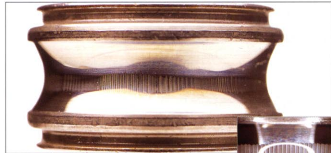
Photo 7-15-5 Part: Inner ring of a deep groove ball bearing Symptom: Fluting occurs on the raceway surface (High frequency) Enlargement
