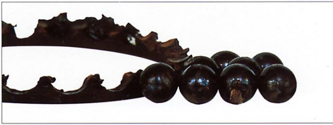
Photo 7-14-5 Part: Balls and cage of Photo 7-14-3 Symptom: Cage is damaged by melting, balls become discolored and melted Cause: Excessive preload
