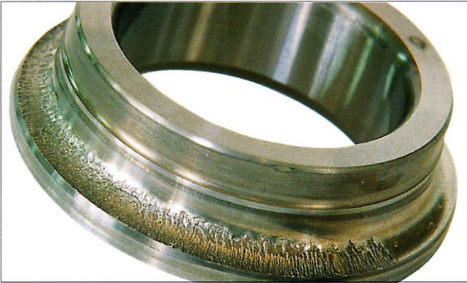
Photo 7-1-1 Part: Inner ring of an angular contact ball bearing Symptom: Flaking occurs around half of the circumference of the raceway surface Cause: Poor lubrication due to entry of cutting coolant into bearing
