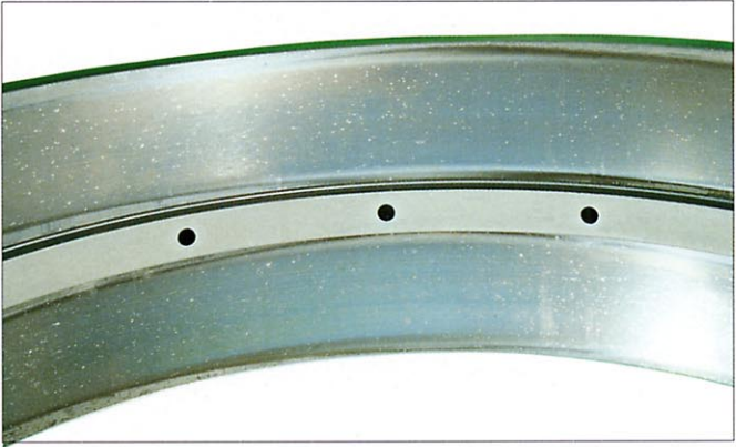
Photo 7-8-2 Part: Outer ring of a double-row tapered roller bearing Symptom: Indentations on raceway surface Cause: Debris caught in the surface
