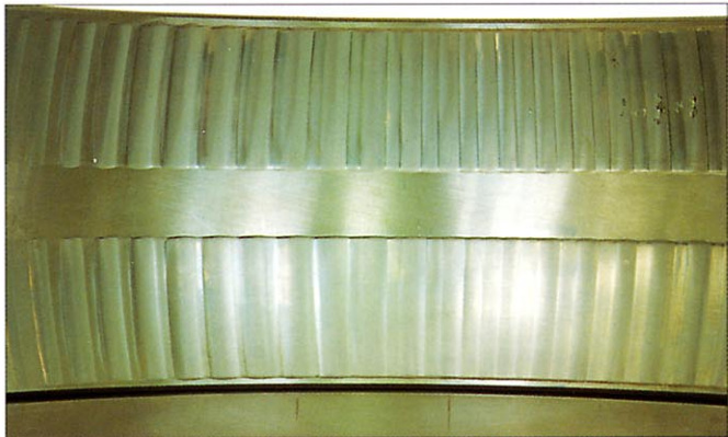
Photo 7-10-2 Part: Outer ring of a spherical roller bearing Symptom: Wear having a wavy or concave-and-convex texture on loaded side of raceway surface Cause: Entry of debris under repeated vibration while stationary
