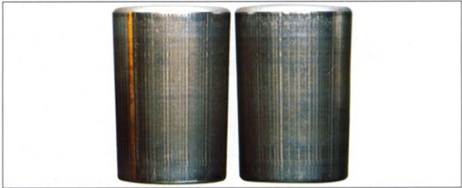
Photo 7-15-2 Part: Tapered rollers in Photo 17-15-1 Symptom: Striped pattern of corrosion occurs on the rolling surface
