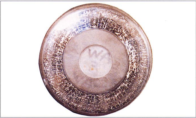
Photo 7-6-2 Part: Roller of a tapered roller thrust bearing Symptom: Thermal cracks occur at large end face of roller Cause: Heat generation due to sliding with the inner ring rib under poor lubrication
