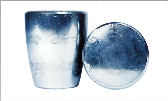
Photo 7-3-6 Part: Convex rollers of Photo 7-3-5 Symptom: Scoring on the roller end face Cause: Debris, which is caught in surface, and excessive axial loading
