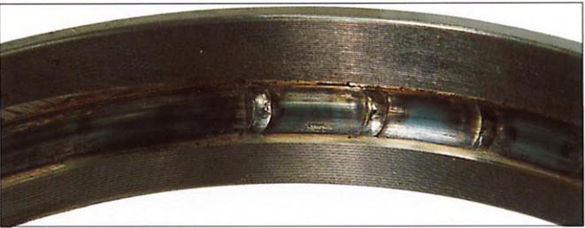
Photo 7-14-4 Part: Outer ring in Photo 7-14-3 Symptom: Raceway discoloration, melting occurs at ball pitch intervals Cause: Excessive preload
