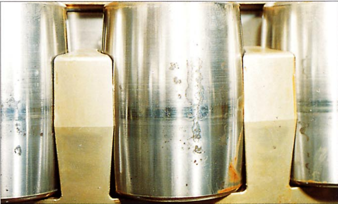
Photo 7-16-4 Part: Rollers of a spherical roller bearing Symptom: Pit-shaped rust on rolling contact surface. Corroded portions. Cause: Moisture condensation during storage
