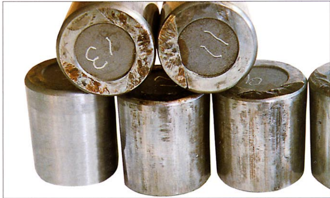
Photo 7-10-4 Part: Tapered rollers of Photo 7-10-3 Symptom: Stepped wear on the roller head end face Cause: Fretting progression due to excessive load while stationary
