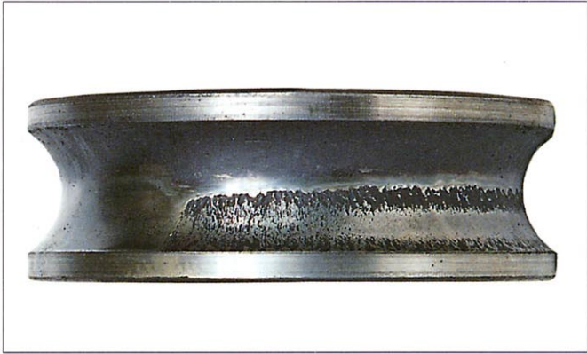
Photo 7-1-2 Part: Inner ring of an angular contact ball bearing Symptom: Flaking occurs diagonally along raceway Cause: Poor alignment between shaft and housing during mounting
