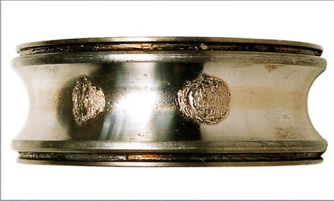
Photo 7-1-3 Part: Inner ring of deep groove ball bearing Symptom: Flaking of raceway at ball pitch Cause: Dents due to shock load during mounting
