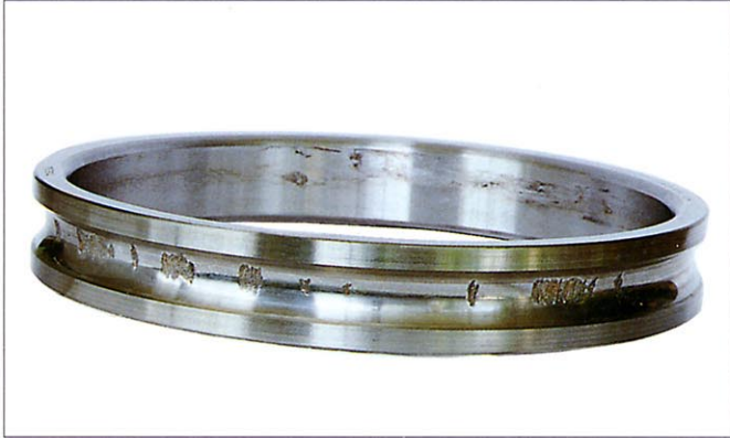
Photo 7-1-4 Part: Inner ring of an angular contact ball bearing Symptom: Flaking of raceway at ball pitch Cause: Dents due to shock load while stationary
