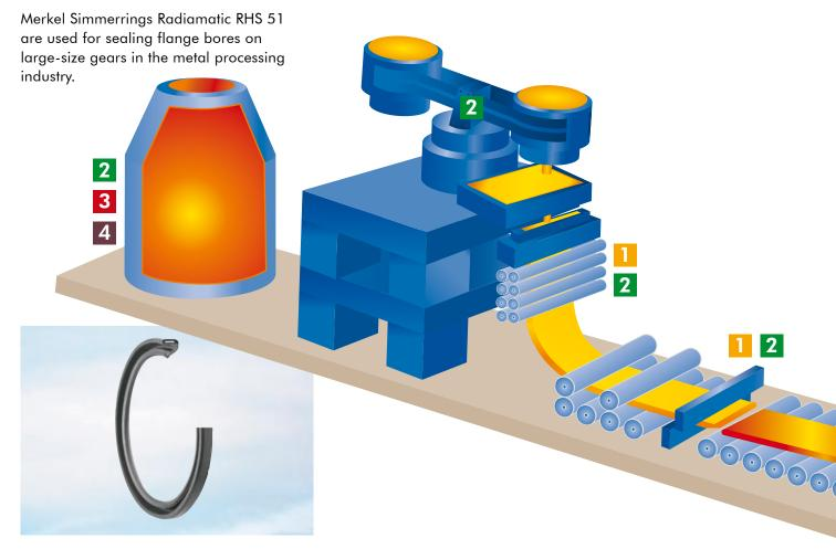
Two functionally adapted elastomer components and an integrated steel strip ensure a high level of functional reliability.
